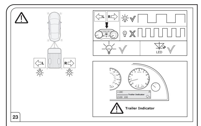
The following lamp functions for the trailer are not supported by all towing vehicles with DRL circuit:
