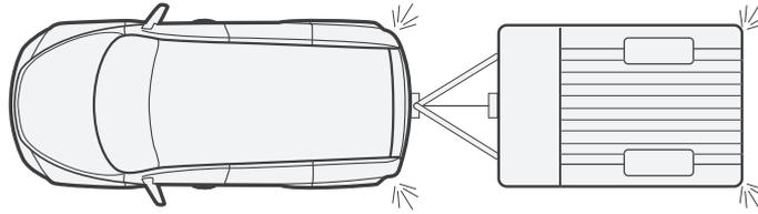
2x Fog lamps on Vehicle then 2x Fog lamps on trailer needed
