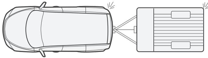
1x Fog lamp on Vehicle then 1x Fog lamp on trailer needed
