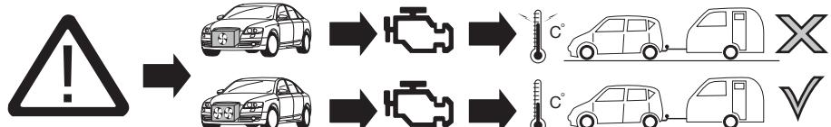
**ATTENTION!** The vehicle's cooling capacity may have to be increased when retrofitting a trailer coupling!
