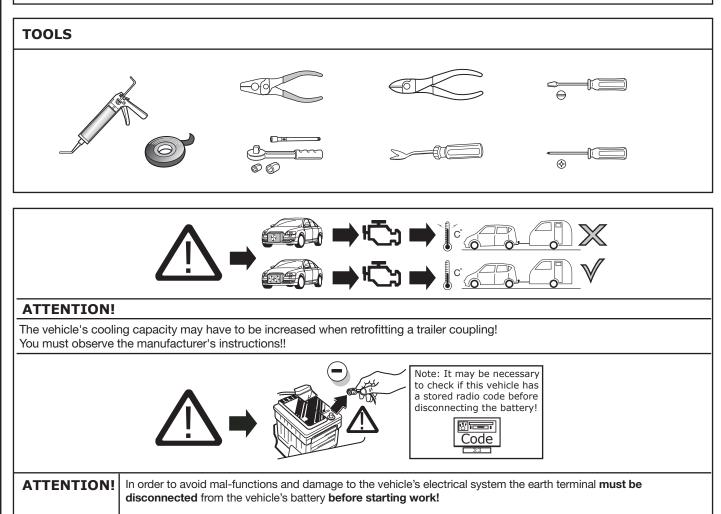
Both the trailer module and the vehicle's control unit for the electrical system can be damaged during work on the data bus connections if the battery is not disconnected!
